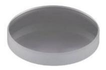
1-25. Ø 25.0 mm UVFS Aspheric Lens, f = 20.0 mm, NA = 0.65, Uncoated
