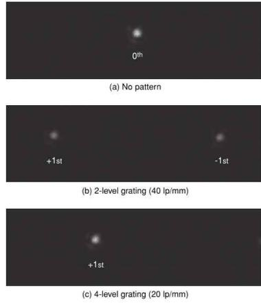
Figure 4: Diffraction efficiency (typical example)
