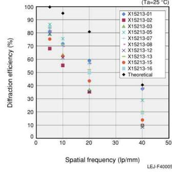
● High linear phase modulation characteristics
